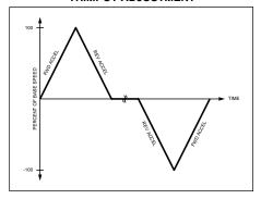
output (RACC also sets the forward deceleration time). To increase the reverse acceleration time, rotate the RACC trimpot clockwise. To decrease the reverse acceleration time, rotate the RACC trimpot counterclockwise.
