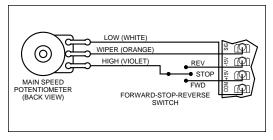
side of the switch to the -15V terminal, as shown in Figure 10. Rotating the Main Speed Potentiometer clockwise will increase motor speed in the direction selected by the switch. Rotating the Main Speed Potentiometer counterclockwise will decrease motor speed. **Note:** Jumper J5 must be set to the "15V" position.
