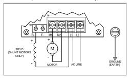
**Note:** Do not connect motor armature leads to F1 and F2 quick-connect terminals. Do not use F+ and F- terminals of Terminal Block TB2 for any purpose other than to power the field of a shunt wound motor.
