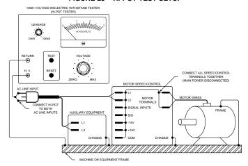
FIGURE 28 - HI-POT TEST SETUP
